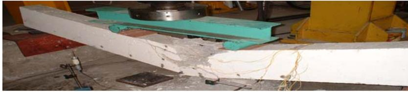
Plate 1. Failure mode of beam A1 (Control beam)
