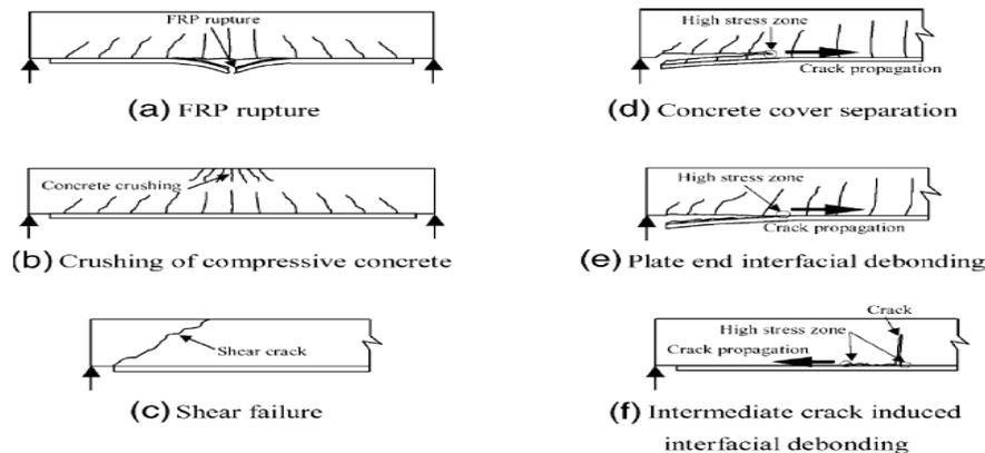
Figure 1: Failure modes of strengthened beams [16]
