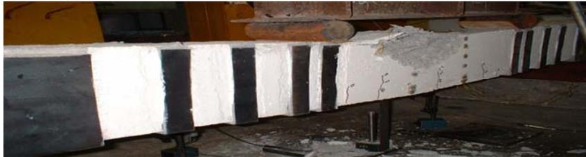
Plate 2. Failure mode of beam B4 (steel plate strengthened beam with L shape end and intermediate anchorages)
