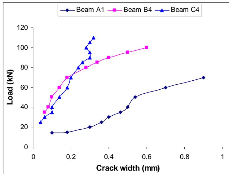
Figure 6: Behaviour of crack width of intermediate anchored strengthened beams
