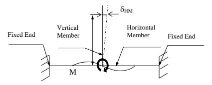
Figure 4: Horizontal member subjected to bending moment
