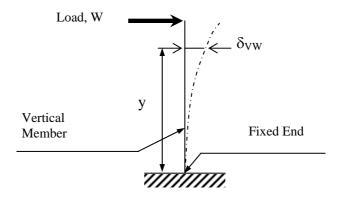
Figure 2: Vertical member as a cantilever
