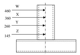
Figure 5: Location of points for experimental testing (All dimensions in mm).
