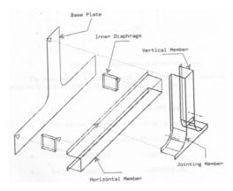
Figure 1: Parts of specimen
