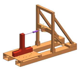
Figure 6: The in-plane bending experiment on the test rig.
