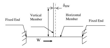
Figure 3: Horizontal member subjected to axial load, W
