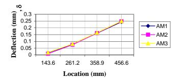
Figure 15: Deflection of vertical member and joint region of continuous sill member (Unit: mm)
