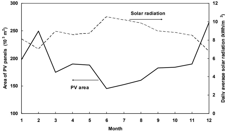
Fig. 2. Area of PV panel system required, around the year, to run the air compressor.
