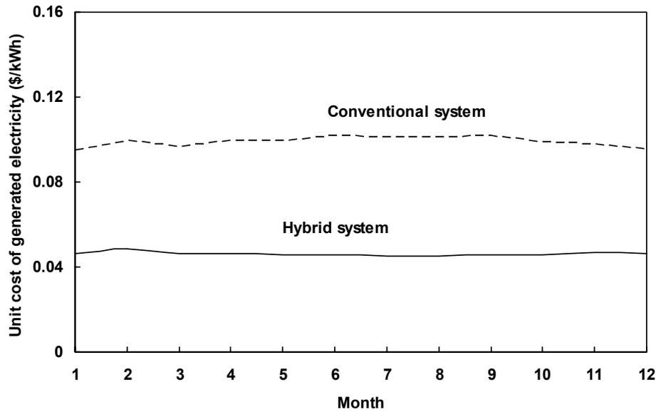
Fig. 5. Unit prices of generated electricity by conventional GT and PV hybrid system.
