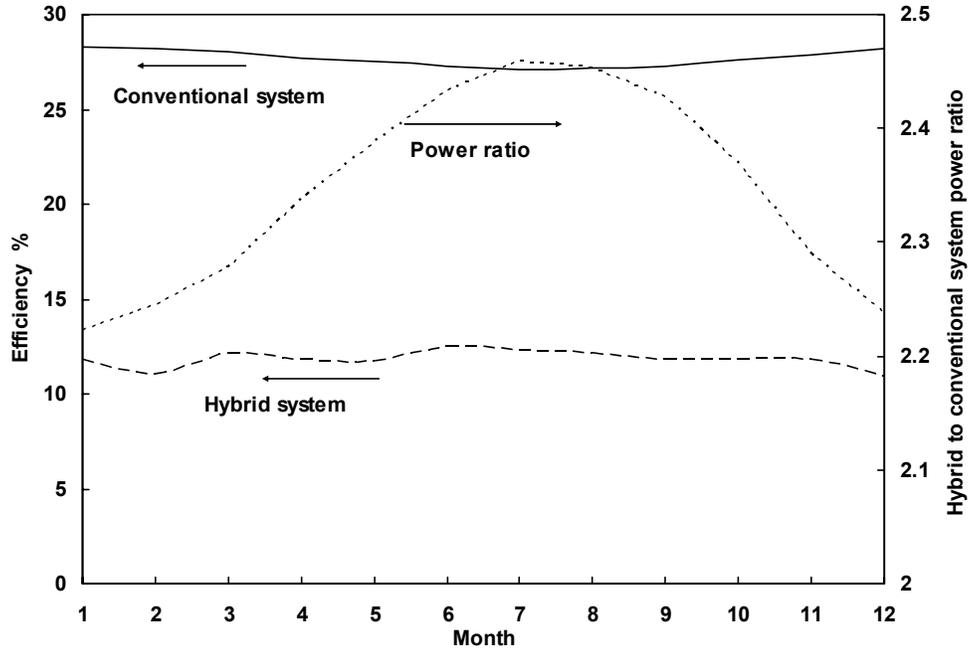
Fig. 3. Efficiencies and power ratios of a conventional GT and a PVGT system.
