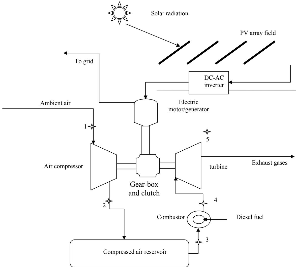
*Fig. 1. The proposed PV-Gas turbine hybrid system.*
