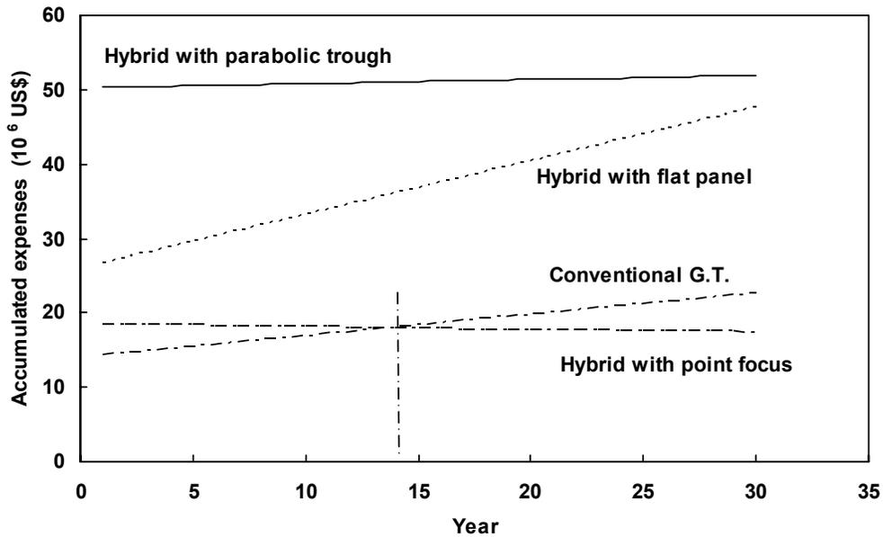
Fig. 4. Accumulated expenses of a conventional GT and three types of PV hybrid systems: flat panel, parabolic trough, and point focus.
