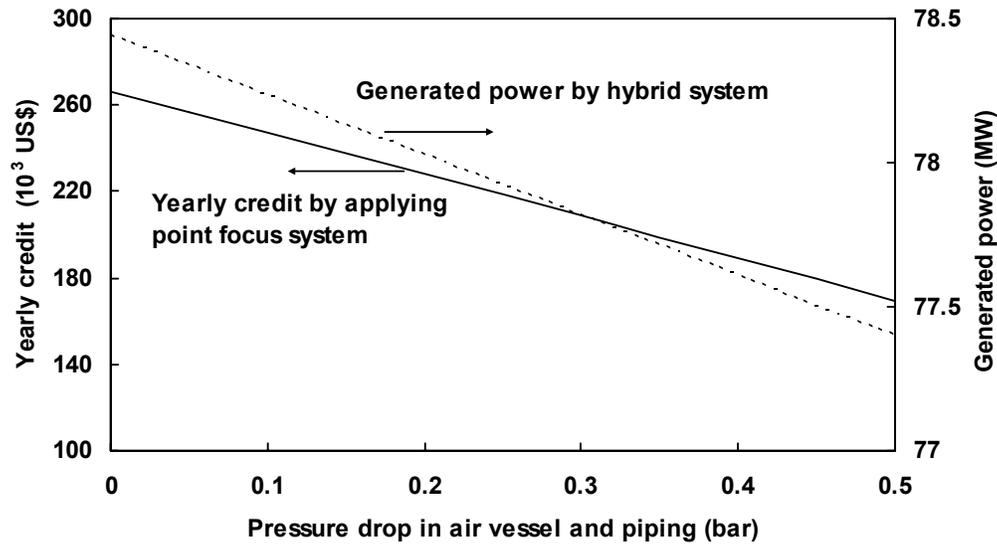
Fig. 6. The effect of pressure drop in the compressed air on the yearly credit and generated power of PV/point focus hybrid system.
